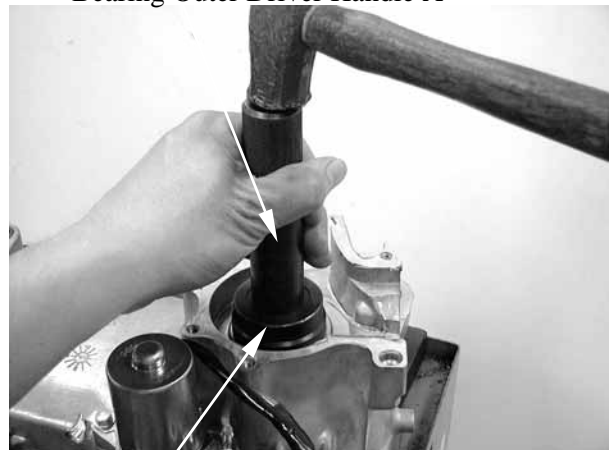
Bearing Outer Driver, 42x47mm Pilot, 20mm
